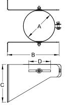
For vent runs passing parallel to a wall, a Wall Support (WS) can reinforce vents that run 3 3/8" to 6 7/8" from the wall to the center of the vent. The wall support can support up to 30' of vent duct.
