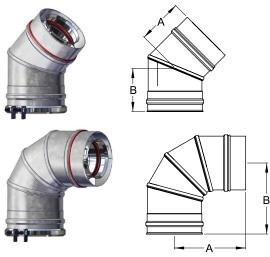
An offset will be required if the vent cannot pass directly above the appliance. EXCELDirect Power Vent<sup>®</sup> elbows are available in 45° and 90°. The outer casing is Galvalume. The stainless steel inner casings are seam welded to ensure there is no leakage. A locking band is included with each elbow.
