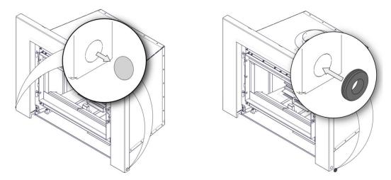
3. Pass the power cord through the opening in the trim. Once the cord is inside the insert, pass it through the round opening in the support leg of the insert and install the strain relief connector in that location. Do not tighten the strain relief connector to the cord at this time.
