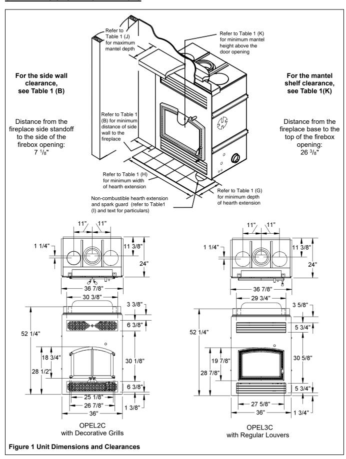
\* WARNING: COMBUSTIBLE FRAMING IS NOT PERMITTED IN THE SPACE DIRECTLY ABOVE THE FIREPLACE. THE ONLY EXCEPTION IS FOR FRAMING USED TO SUPPORT THE FACING MATERIAL AND MANTEL. THE AREA ABOVE THE FIREPLACE MUST BE FREE OF COMBUSTIBLES FOR AT LEAST THE HEIGHT PROVIDED IN TABLE 1(C).
