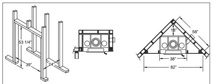
The framing dimensions are larger than required for ease of installation. Examples shown here are for a Louvered OPEL+ C. An extra 12" is required on the left of the fireplace of a Clean Face OPEL+ C to connect the intake air duct. The Heat Dump Option will also require an extra 12" on the selected side.
