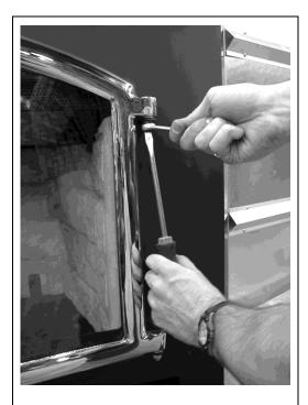
**Figure 6 Door Hinge Adjustment**
