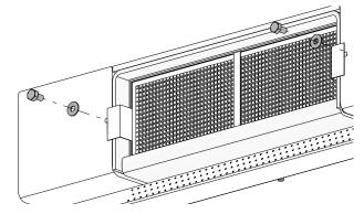
Wrap the new catalyst on all sides with the catalyst gasket. Enough gasket is supplied to wrap the catalyst with two layers of the gasket material. Carefully insert the catalyst and catalyst support plate into the opening and reinsert all four screws that hold it in place. The catalyst gasket expands as it is heated; so, it is normal for the gasket to have some small gaps after being inserted. As the gasket expands, the spaces will be filled.
