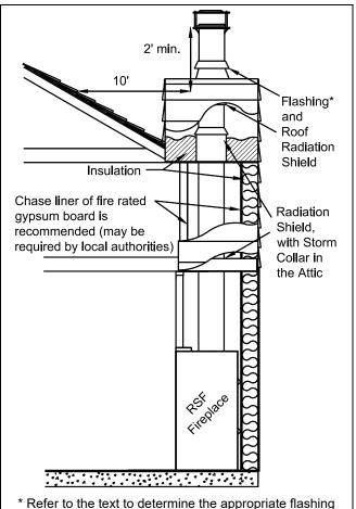
Figure 17 Chimney Installed with a Chase **Enclosure Example**
