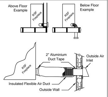
Figure 13 Outside Air Connection and Installation Example
