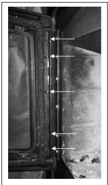
Figure 7 Hinge Adjustment on the Door
