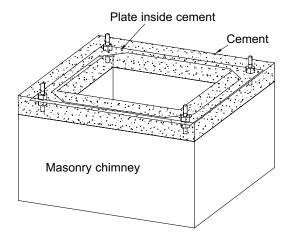
3. You can install the anchor plate damper once the cement is dry. Place the insulation pad provided over the protruding bolts making sure the hole in the pad is centered. Place the anchor plate damper over the bolts and the insulation pad with the damper rod in the direction you plan to use it. Tighten the nuts to fasten the anchor plate damper in place. Make sure the nuts are tight enough to firmly compress the insulation pad.
