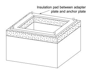
4. Build your masonry wall until you reach the damper rod height. Slide the ferrel on the rod until the keyed plate touch the masonry wall. The flat part welded to the ferrel must point down. Locating the ferrel guide in a brick (or stone) joint will ease the installation.
