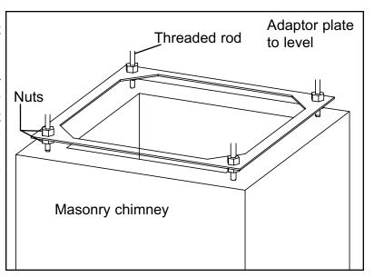
2. Pour the masonry on the top of the adapter plate. Make sure the adapter plate it is kept level and well centered with the chimney until the masonry has set.
