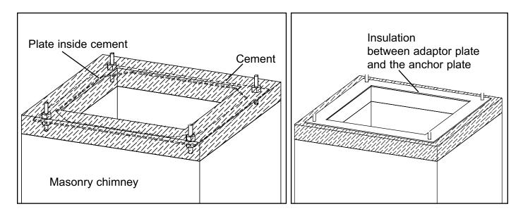
3. You can install the anchor plate damper once the masonry is dry. Place the insulation pad provided over the protruding bolts making sure the hole in the pad is centered. Place the anchor plate damper over the bolts and the insulation pad. Tighten the bolts to fasten the anchor plate damper in place. Make sure the bolts are tight enough to firmly compress the insulation pad.
