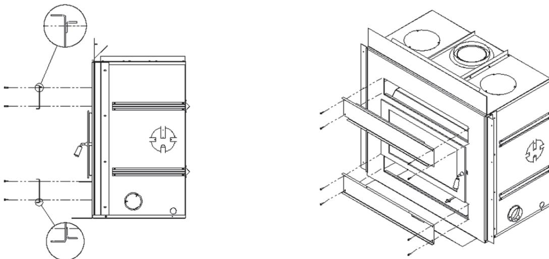
Figure 5 Mounting brackets installation
