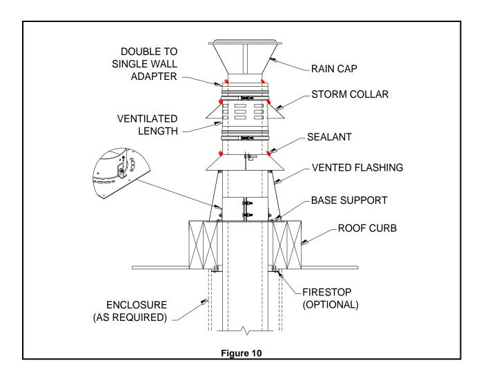
10. Put the rain cap over the Ventilated Length and push the Closure Ring onto the Ventilated length before installing the Locking Band. The Rain Cap comes with its own Closure Ring and Locking Band.
