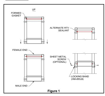
To connect two parts together simply insert the male end of one part into the female end of the adjoining part and press firmly until the outer casings are fully inserted one into another. Once the parts are firmly joined, install a locking band over the outer casing joint as shown in **Figure 1**. A locking band comes with every part. You can put a small amount of liquid dish soap on each gasket to make it easier to assemble the vent. Do not use a petroleum-based lubricant.
