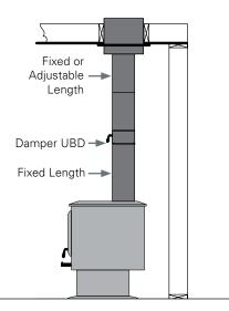
**STRAIGHT UP INSTALLATION** For most straight up installations, the only part required is an adjustable length (UBAF). The UBAF adjusts to allow any overall length from 40" to 68".
