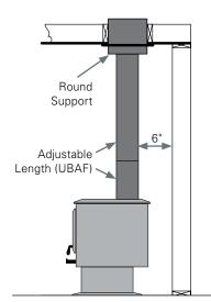
Clearance Between Ceiling & Top Off Elbow 6" Minimum 90° Elbow (UB90) Adjustable Length (UBAF)
