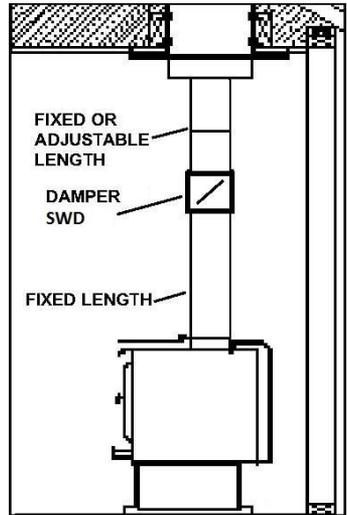
Note: Plan the fixed and adjustable measurements that you will require in advance. Adjustable or slip sections should always be installed above a SWD. A slip section cannot be installed directly onto the SWD.
