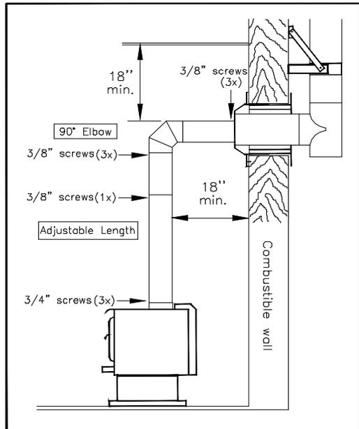
4. Extend the adjustable length up until the 90° elbow reaches the chimney pipe adapter. Screw the elbow to the adapter using the three 3/8" metal screws provided.
