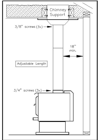
2. Slide the top length of the SWA up over the chimney pipe adapter at the bottom of the chimney support. Connect it to the adapter with three 3/8" metal screws provided.
