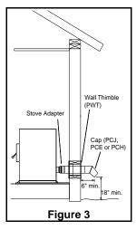
Determine a location for the vent that is as near as possible to the appliance outlet.
