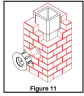
**NOTE**: Any EXCELPellet Stove Adapter component (3PASH, 3PAT4, 3PAT3 or 3PI4) may be used as an alternative to the Universal Stove Adapter (PAS).
