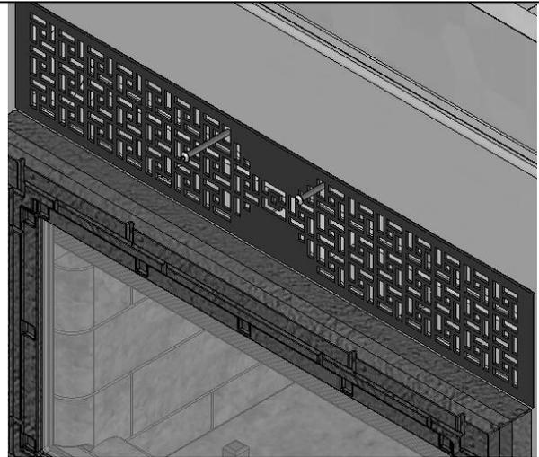
Figure 4 Top louver installation
