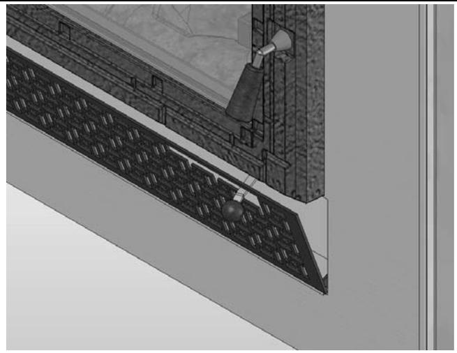
Figure 2 Bottom louver installation
