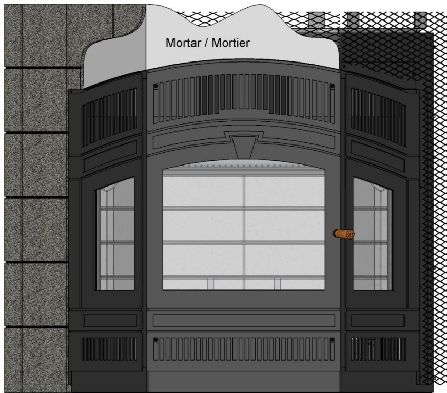
Figure 2 Facing with masonry
